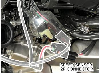
Mhen installing main unit, protect by rolling up attached sponge.
