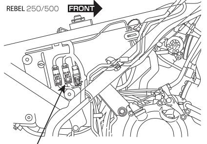
Tightening together with other ground terminal
