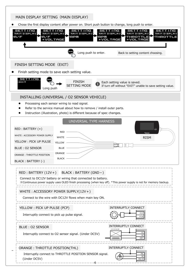
HOW TO INSTALL (i-Map installed vehicle HONDA MINI HEATER LESS O2 SENSOR MODEL)
