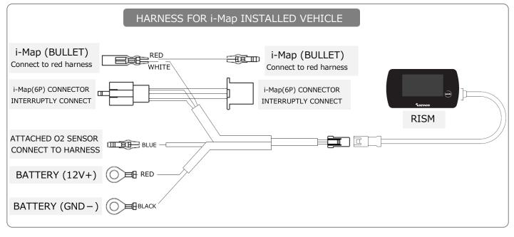
• Interruptly connect to stock O2 sensor connector. Please use same shape connector according to the vehicle.
