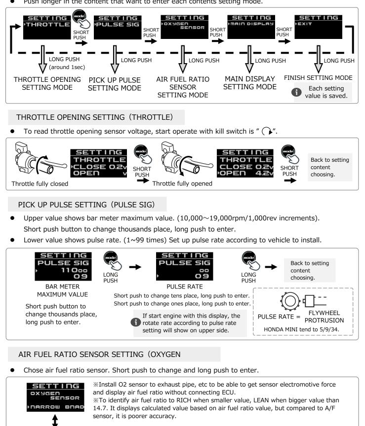
X"WIDE BAND" is supposing that with LAF sensor which is chosen by HONDA MONKEY125 (8BJ-JB03), CT125 (8BJ-JA65), etc. The LAF sensor of specified vehicle is basically unable to use as air fuel ratio measurement because it decides operation automatically by electronic control.
