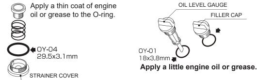
**Tighten with specified TORQUE!**
