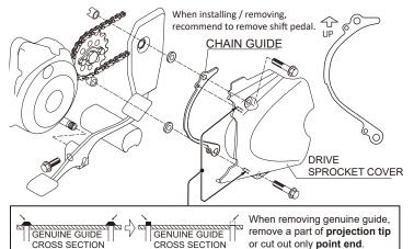
※This product is not to protect the interface of drive chain, crank case, etc. If the drive chain is not stable, adjust tension regularly.
