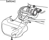
1-2 Remove Fuel drain hose and crank case breather hose from air cleaner case.
