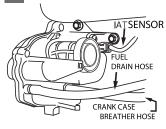
1-3 Tighten the fuel drain hose to the harness, etc with tie wrap.
