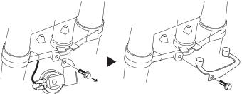
Remove horn & wire connector Make insulation treatment on wire connector not to interfere when driving.
