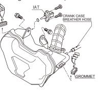
POINT : FI setting is not required in case of stock engine and Kitaco JMCA muffler combination. oBasically, reuse stock parts if it is unattached. If there is a hard degradation like a blem,
