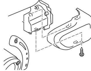
**2** Remove intake air temperature sensor (IAT), fuel drain hose and crank case breather hose from air cleaner case.
