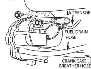
**3** Tighten the fuel drain hose that was removed from air cleaner case with sensor harness by tie wrap.
