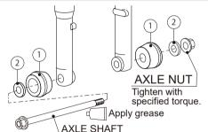
Axle nut is lock nut structure. Once tighten nut to axle shaft, axle shaft screw and nut surface might peel off. There is no problem with the quality.
