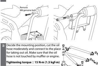
Add engine oil (standard amount + 75~100cc) for oil cooler capacity.
