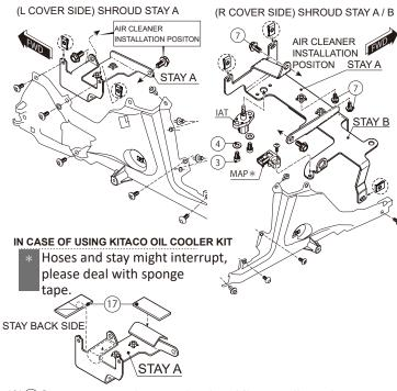
\*To Sponge tape is attached to Kitaco oil cooler kit (frame mounting type).
