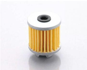
Apply engine oil to O-ring.
