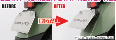
This license plate stay allows you to tilt the license plate installation angle.
