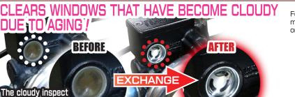
For replacing the inspection window ( $\phi$ 18) of the master cylinder. Replace it when it becomes cloudy or dirty due to UV rays, scratches or aging.
