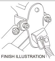
8 ,Put the under cover, bolt, side cover (L) back. Tighten tapping screw and clip trim to finish intallation.
