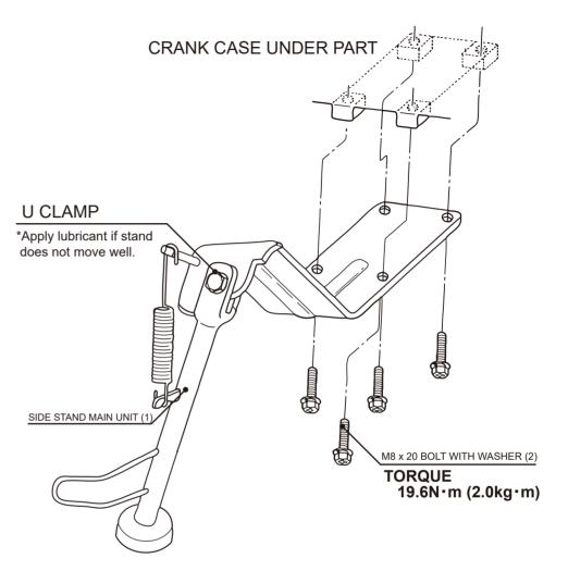
Install side stand main unit (1) to engine crank case under part 4 holes with M8 x 20 bolt with washer (2).
