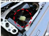
Open tandem seat, remove 6P waterproof coupler cap inside the connector cover.
