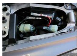
Connect Power Supply Extract Harness with waterproof coupler. Connect your favorite electric parts such as USB supply with ACC  $\oplus$ , GND  $\ominus$ .
