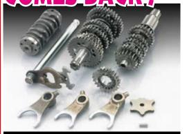
Changes from stock 5 speed to 6 speed to close ratio between each gear. For smoother shifting to keep better power band for sport riding. Reduces friction loss for lightweight for race use.
