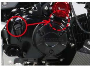
Engine No. JC61E-1304744 $\sim$  is not usable as engine oil inlet has been changed from  $\bigcirc$  to  $\bigcirc$ .
