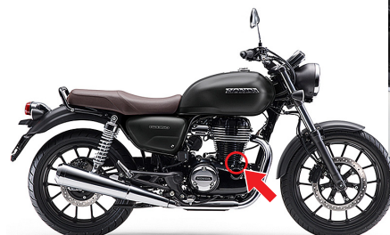
One point dress up with machined aluminum oil filter cover designed with air cooling fins.
