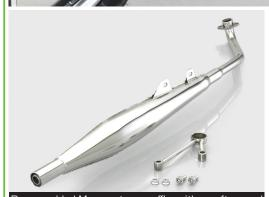
Press-molded Monaca type muffler with a soft curved surface of old Cub style. Torque can be improved over the entire area, and over-rev characteristics with little drop in peak power are achieved.
