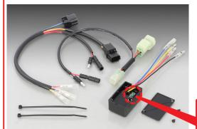
Corrects speedometer error display when changing sprocket teeth. Just insert it between stock coupler. No wiring mods required.
