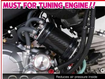
the crankcase through case breather to reduce power loss and temperature increase
