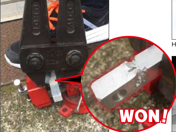
20mm SQUARE ARM is adopted with HDR-LIGHT2010 . Very difficult even to pinch with the special theft arm. * Special cutting tool is used for the test because thefts happens at night silently.
