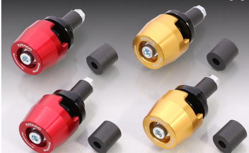
Aluminum machined with bearing built-in!!
