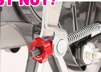
Aluminum machined brake adjust nut with alumite finish newly released!! Dress-up rear brake rod end!!
