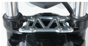
Machined stabilizer has not only dress up effect but also keep the stiffness & save the weight!!
