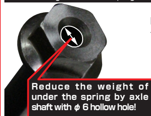
Lightweight axle shaft has hollow hole with \phi 6 to reduce the weight of under the spring.
